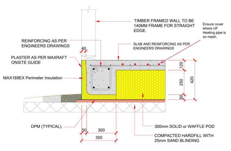
MAXRaft OR MAXRaft Plus+ 420mm Detail
